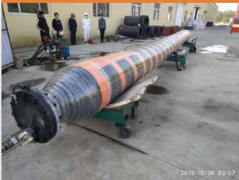
TESTING PRESSURE 22.5 BAR
